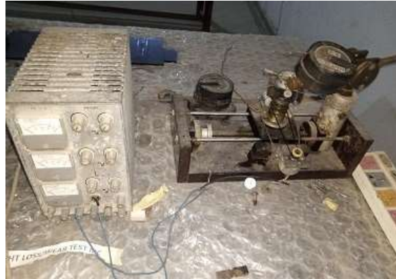
Figure 3: Wear Abrasion Test machine
