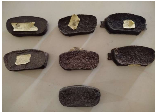
Figure 2: Cow horn reinforced brake-pad samples
