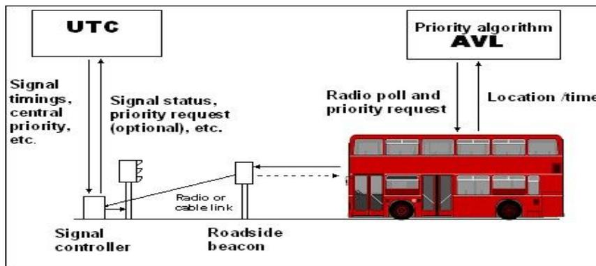
Figure 3. AVL based bus priority architecture in London
