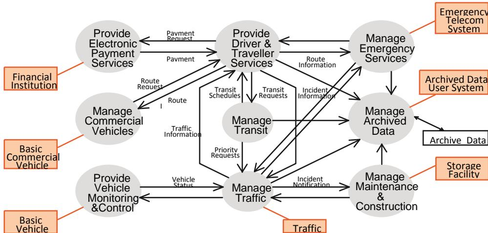
Figure 2 Very High Level Logical Architecture of the U.S. National ITS Architecture (DFD)
