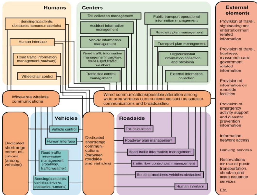
Figure 1: Subsystem Interconnect Diagram from Japanese Physical ITS Architecture
