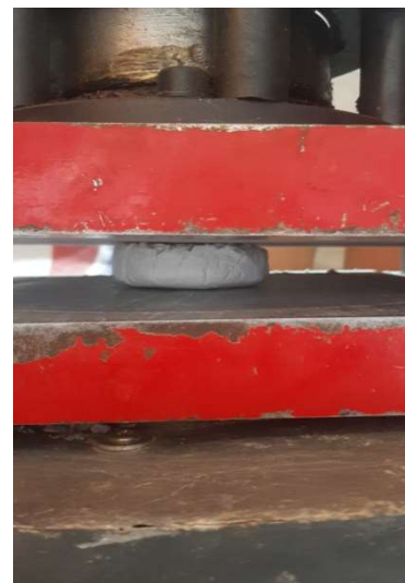
Plate 6: Sample loaded to the press jaws
