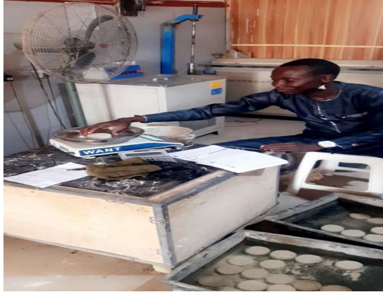
Plate 3: Samples being weighed to determine porosity
