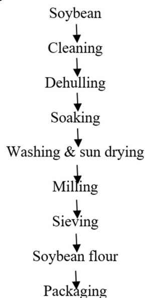
Fig.3.2: The flowchart for the preparation of soybean flour (Ngoddy et al. , 1985).
