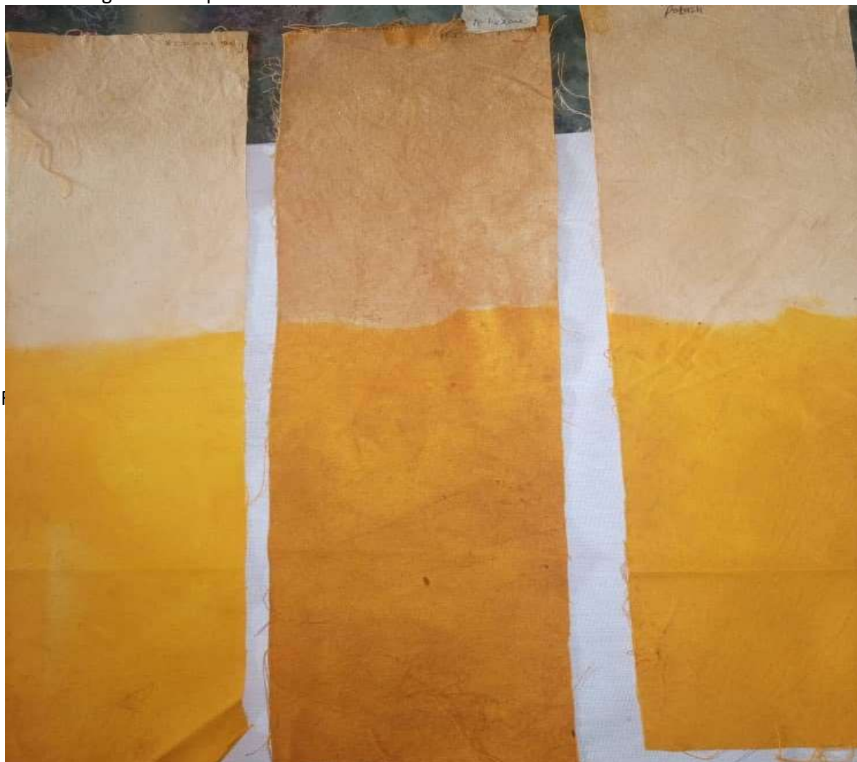
Plate 3: Light fastness of microwave extracted turmeric dye extracted with n-hexane on cotton fabrics using alum and potash as mordants
