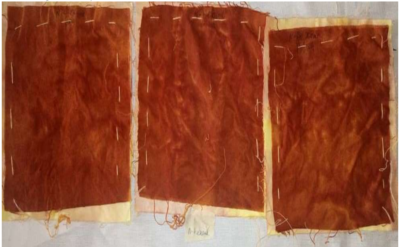
Plate 6: Wash fastness of microwave-extracted turmeric dye extracted with n-hexane on cotton fabrics using alum and potash as mordants
