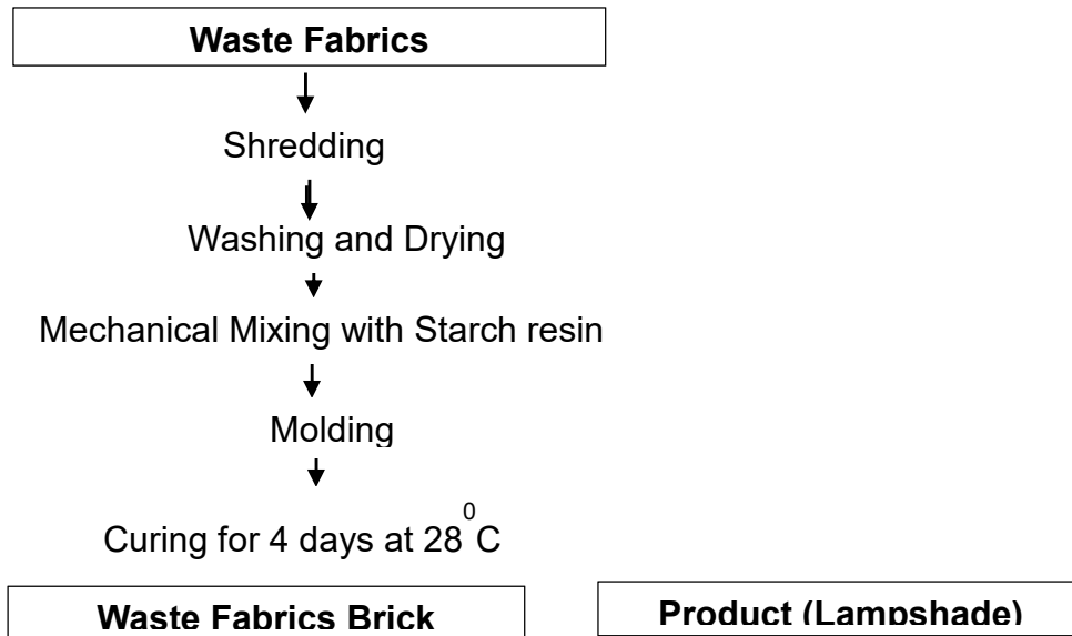
Figure 1: Flow chart for development of ecological bricks and lampshade from fabric wastes and discarded garments
