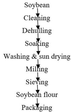
Fig.3.2: The flowchart for the preparation of soybean flour (Ngoddy et al. , 1985).
