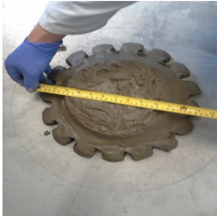
Figure 4.2 The effect of FA concentration on the flow of SCC in presence of 2% of SP.
