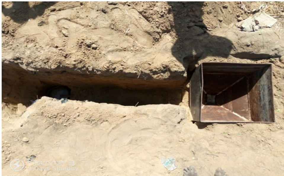
Plate 1: Installation of a Lysimeter
