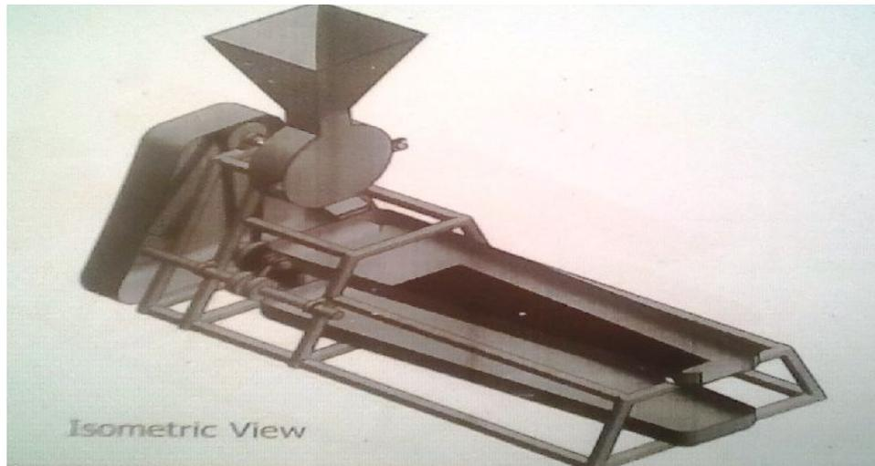
Figure 3a: Isometric View of the Machine
