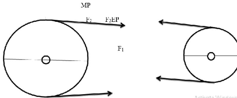
**Figure 2: Impacted forces by the belt**
