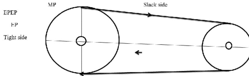
**Figure 1: Tight and slack sides of belt tension**
